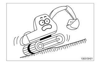
Operate the machine after making ground flat when operation is required on a slope.
